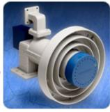
feedhorns feature Chaparral's patented probe for C-Band, reception and a unique low-loss dipole antenna for Ku-Band reception. The dipole is virtually invisible to the C-Band probe, resulting in superior C-Band performance while improving Ku-Band illumination. Both the probe and the dipole are controlled by a Chaparral servo motor, providing infinite skew adjustments and quick selection of horizontal and vertical poles.
